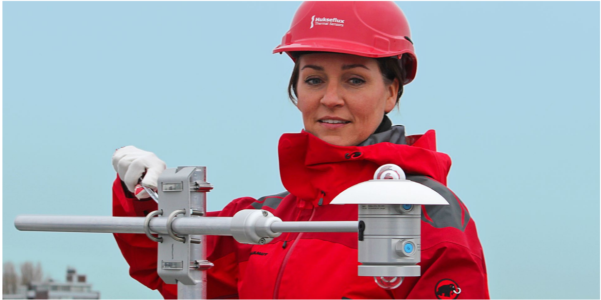
Figure 3.4.3 Installation of an albedometer mounted with AMF02 albedometer mounting fixture and levelled with ALF01 albedometer levelling fixture. The crossarm mounting fixture, connecting the cross arm to a vertical mast is CMF01
